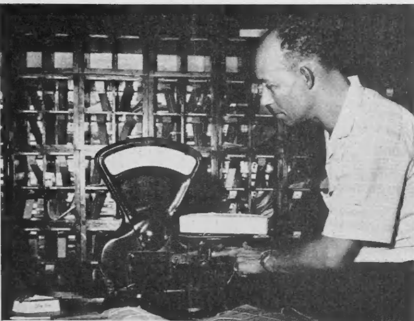
AT THE Concrete Plant, a truckload of rock is weighed on the kilogram scale. This protects both the supplier and the buyer, Lago. It is one of the few instances at Lago when metric weights are recorded. Avoirdupois weight is normally used.
